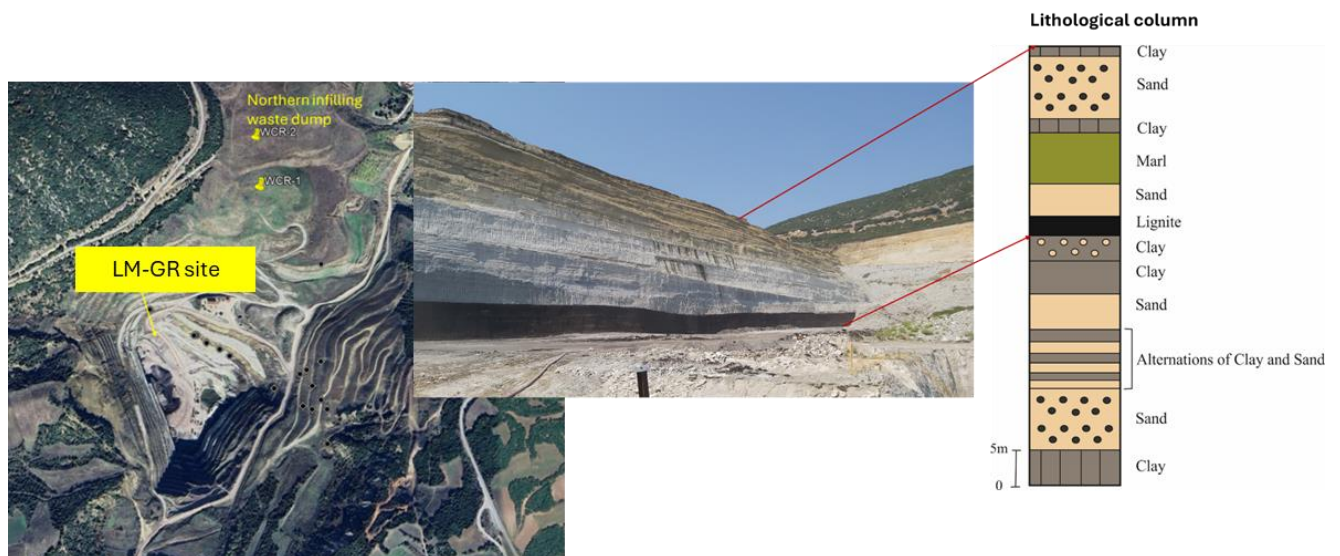
Fig. 5. Location and borehole profile at LM-GR site.
